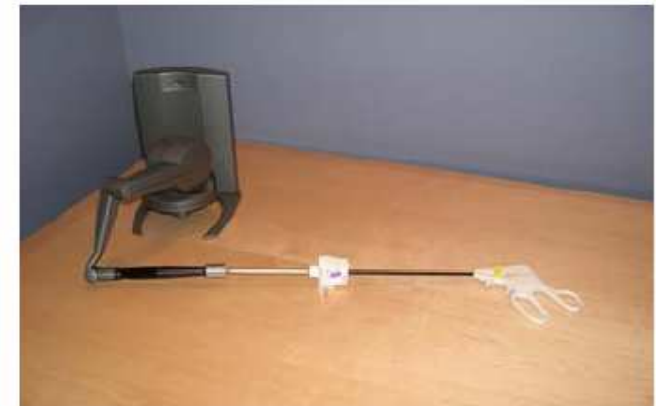
The PHANTOM Desktop haptic device with the Auto Suture® 5mm Endo Clinch® II device attached.
